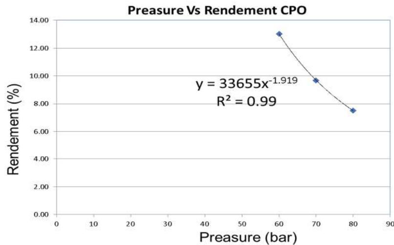
Figure 3. Relationship between pressure and oil loss.
