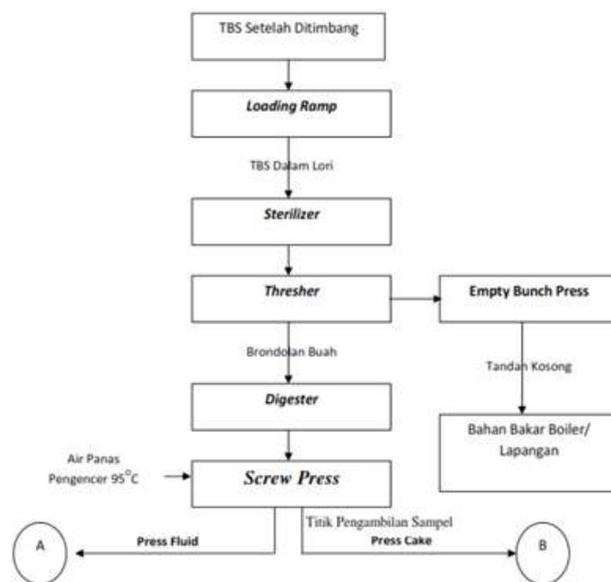
Figure 2. Palm oil processing flow diagram.
