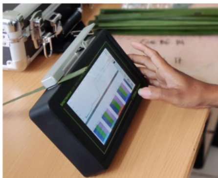
Figure 2. SpectraVue CI-710s leaf spectrometer
