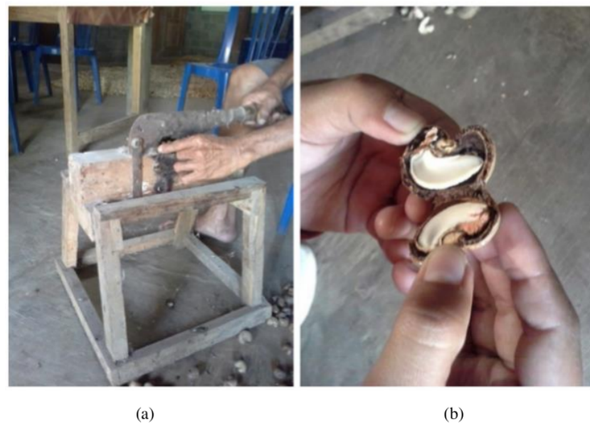
Figure 4 (a) Stripping Tools, (b) Cashews that have been Peeled Source: documentation's author, 2015
